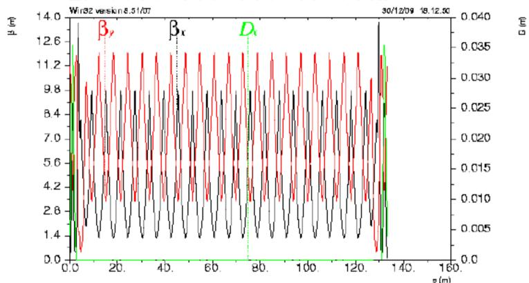
The straight sections are dominated by the 6m FODO cells for the wigglers
