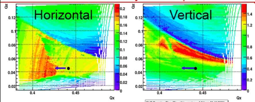
Tune scan simulation to determine optimum working point
