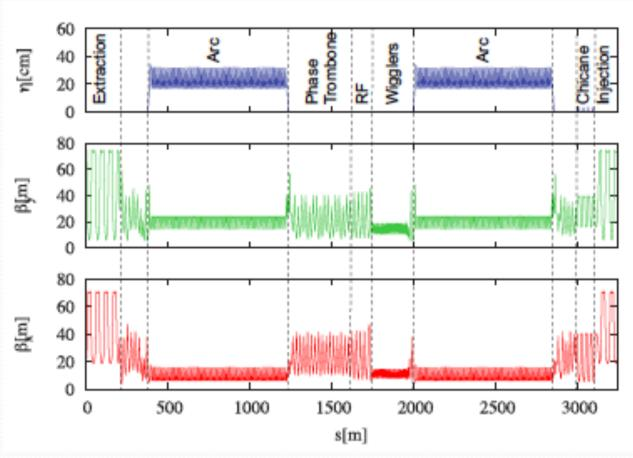
RF is upstream of wigglers in both rings to avoid damage from synchrotron radiation
