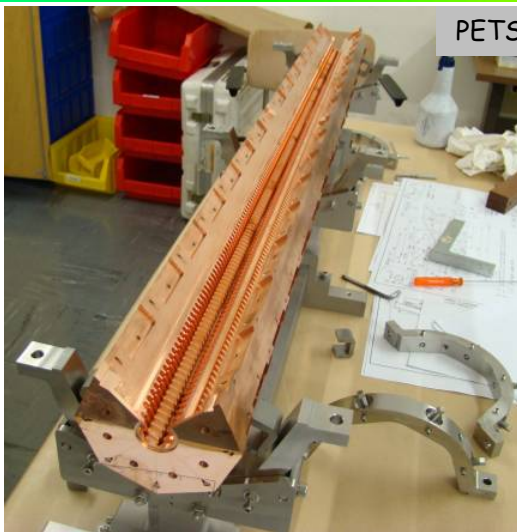
PETS equipped with the power couplers and electronic ruler with pick-up antenna for the phase advance measurements.
