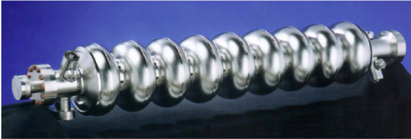
Figure 1.2-1: A TESLA nine-cell 1.3 GHz superconducting niobium cavity.
