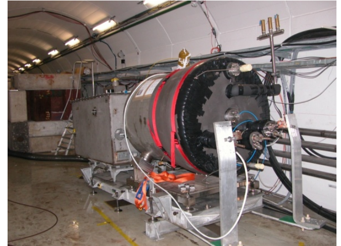
Hg jet in a 15 T solenoid with measured disruption length: ~ 28 cm
