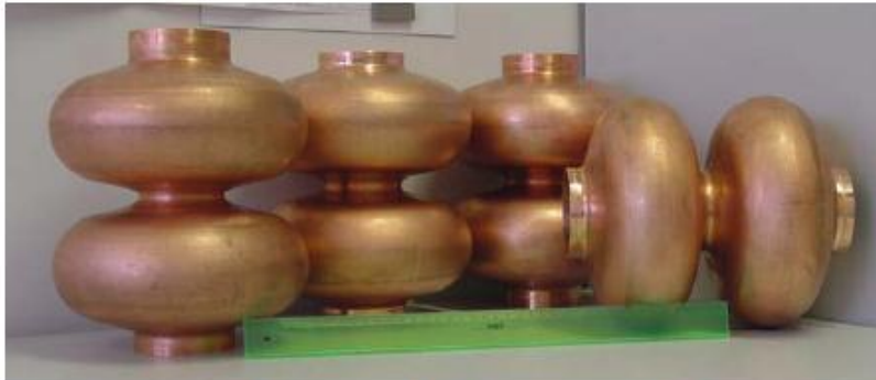
Four double cell NbCu clad cavities produced at DESY from KEK tubes (no cracks on the inside surface)
