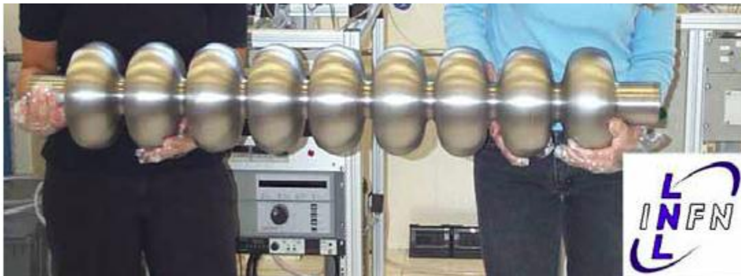
1.3 GHz 9-cell cavity. Damaged after CBP, no test
