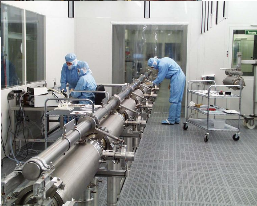
SNS \beta_g=0.61 string at JLab: 3 cavities per string
