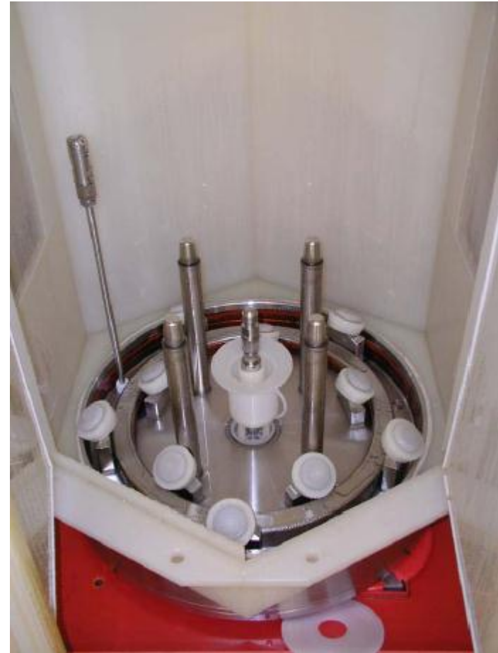
HPR stand inside the clean room at DESY
