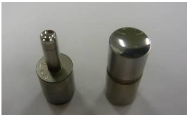
Moulds for DVD optics : 50 nm form accuracy on \varnothing 2\text{ mm} equals ratio of 1 / 40000
