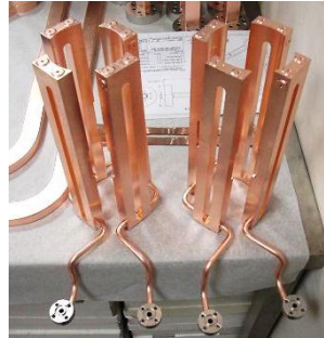
Assembly of cooling circuits
