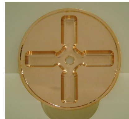
CLIC disk -> series part 2 \mu\text{m} accuracy on \varnothing 80\text{ mm} equals ratio of 1 / 40000
