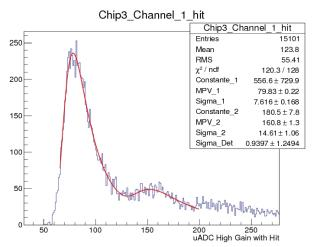
We also fit the second MIP pic, but calculate the convolution of two Landaus is very long ...
