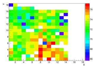
The mean MPV for the dif0 is  $73 \pm 3(4\%) \, uADC$ . From the simulation  $1 \, MIP = 0.095 \, MeV$ .
