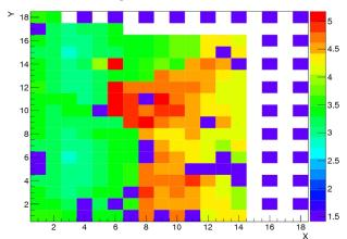
The mean Sigma of the detector for the dif0 is  $3.8 \pm 1(25\%)~uADC$ .
