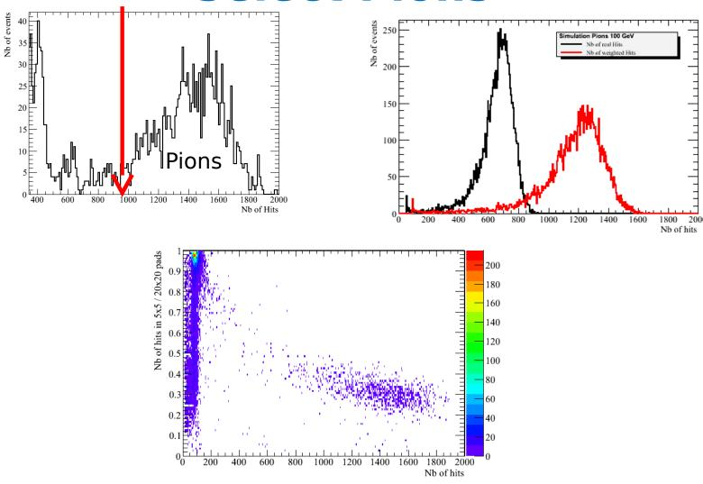
The number of hits in a small core of 5x5 cells compared to a larger core 20x20, must be closer to 1 for  $\mu$  and  $\rho$  and smaller values for  $\pi$
