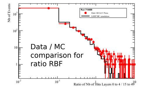
With cut R<0.5 Electron rejection and pion selection efficiency > 95%
