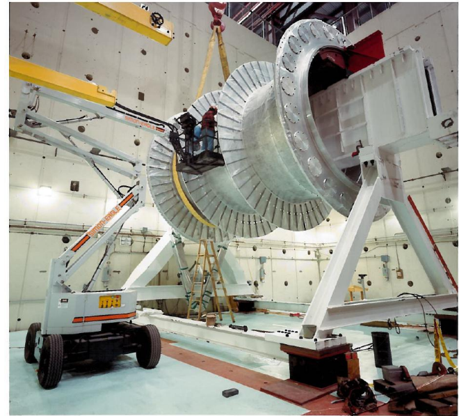
SLD, Liquid Argon Calorimeter Assembly Beam (Option 1)
