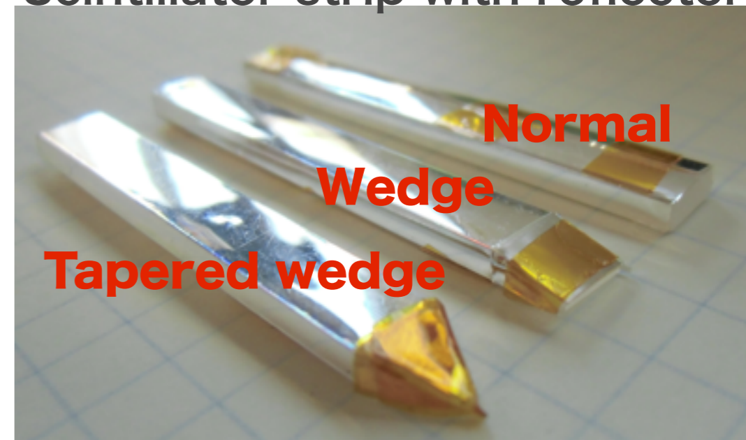
Scintillator strip with reflector
