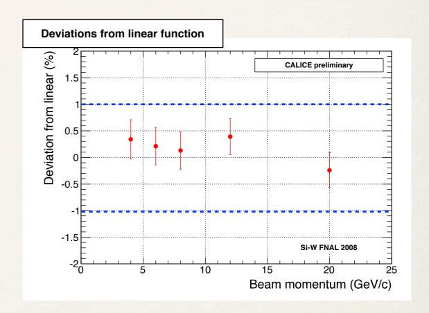
The deviations from linear function are less than 1 %
