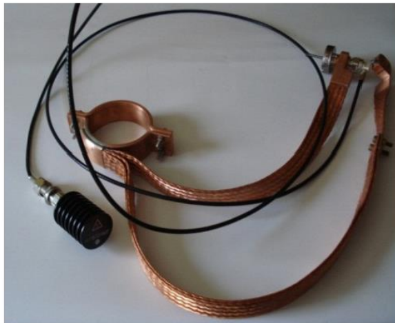
Figure 4: Prototype of the thermal braids for standard TESLA cavities (courtesy NCNR).
