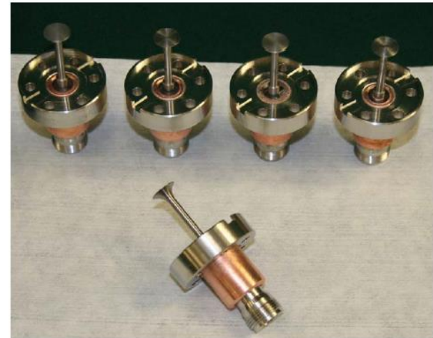
Figure 3: New feedthroughs for XFEL cavities.
