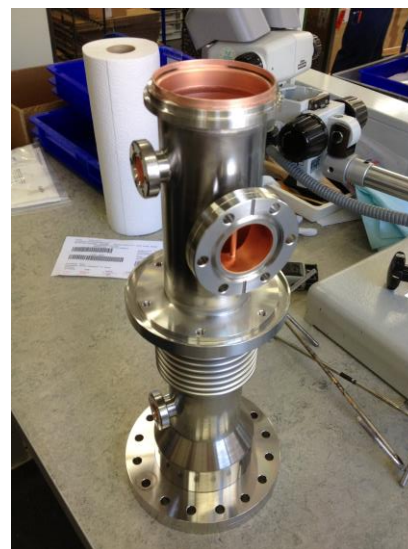
Collini Copper coated warm outer and inner conductor
