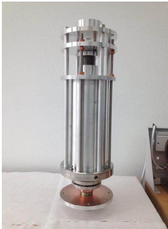
Tool for cold part welding
