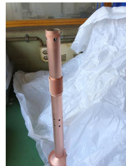
Collini Copper coated warm outer and inner conductor
