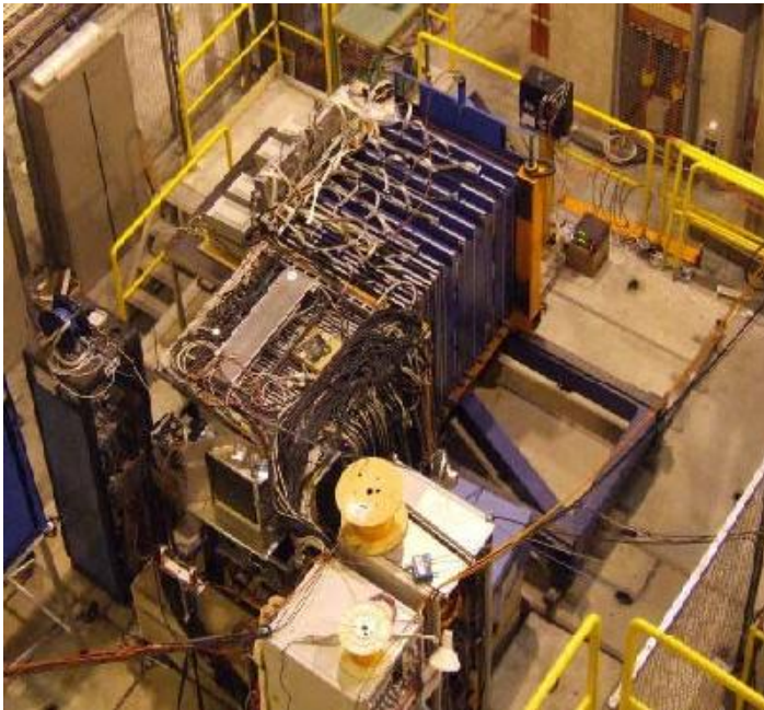
CALICE Test Setup at CERN including Muon System/Tail Catcher
