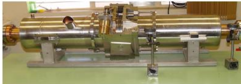
1.3 GHz Prototype Dressed Cavity with Scissors Tuner
