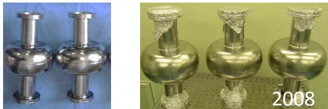
CP 40 MV/m, Q_0 = 1.6 \times 10^{10} @ 2K EP 48 MV/m, Q_0 = 1.0 \times 10^{10} @ 2K
