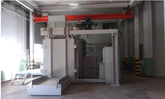
EBW Machine (High Voltage)
