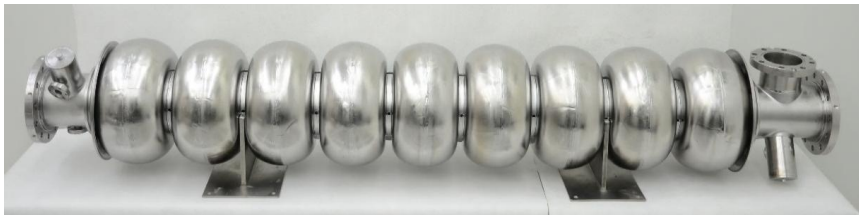
9-cell cavity IHEP-02 (with HOMs, 2012)
