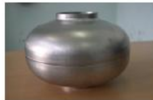
Prototype 1.3GHz cavity Nb half cells welded
