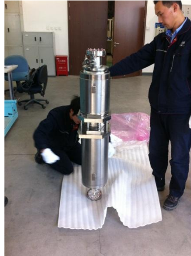
1.3GHz 9-cell cavity (IHEP-01,IHEP-02) IHEP first Large-grain low-loss shape, 20MV/m
