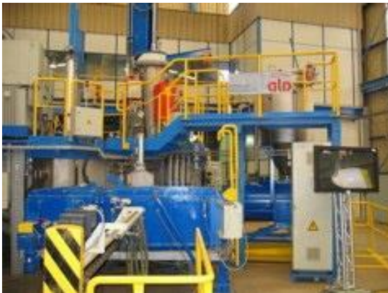
Electron beam furnace for the refinement of Niobium metal, producing 210 tonnes per annum
