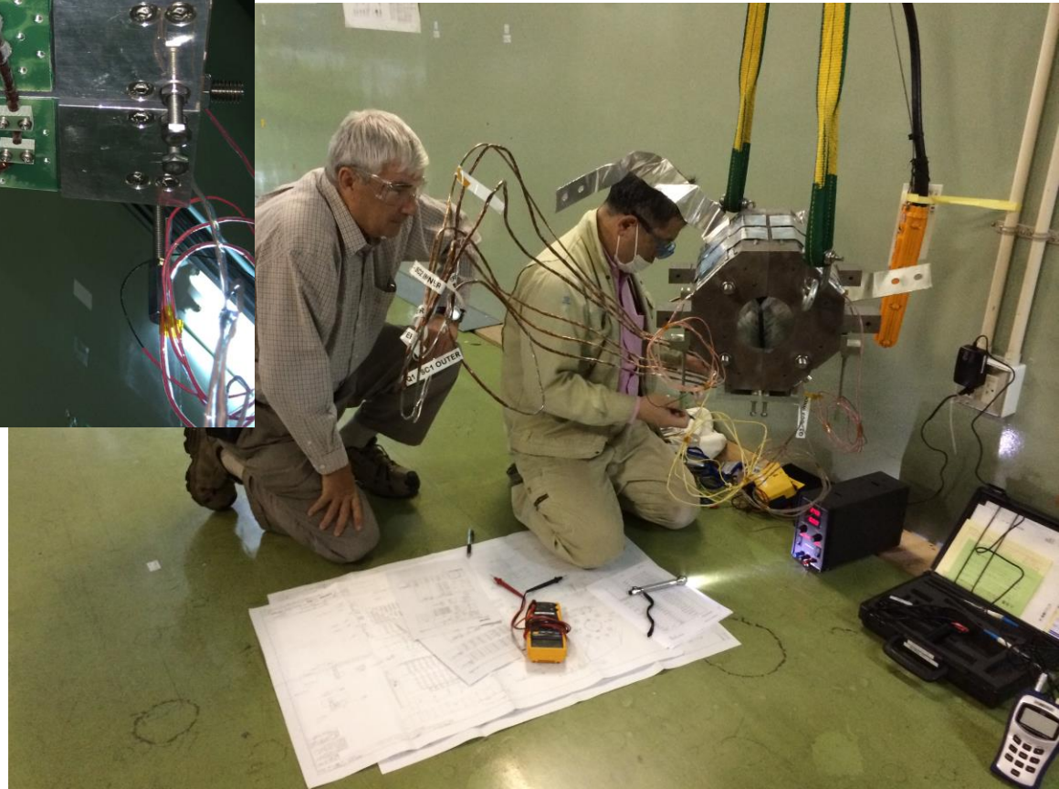
Checking field polarities with Hall probe
