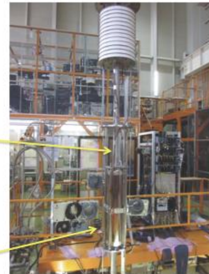
Warm tube and cavity-shield suspended from the cryostat top plate
