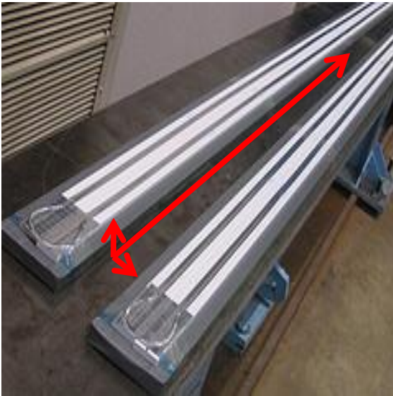
SiD Baseline – long scintillator strips with WLS and SiPM readout
