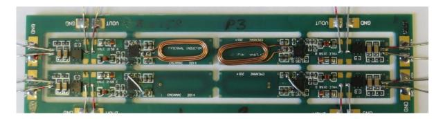
Each Converter PCB 10 mm x 63 mm. Different Coil Configuration Channel D: Embedded Coil with 2 via: 687 nH, 83 m $\Omega$ Channel C: Embedded Coil with 1 via: 703 nH, 83 m $\Omega$ Channel B: External Coil: Wurth 540 nH\* with short Leads Channel A: External Coil: Wurth 540 nH\* with short Leads \* With BK Precision LCR Meter
