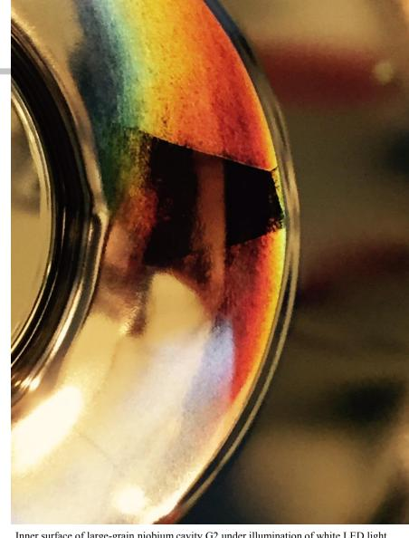
Inner surface of large-grain niobium cavity G2 under illumination of white LED light. The rich color is a result of interference of light when reflected from the near surface of the niobium. An outstanding grain in the middle of picture reflects the light differently due to presumably its unique grain orientation. Test data of cavity G2 are presented in slide #6. Photo credit: Pashupati Dhakal.
