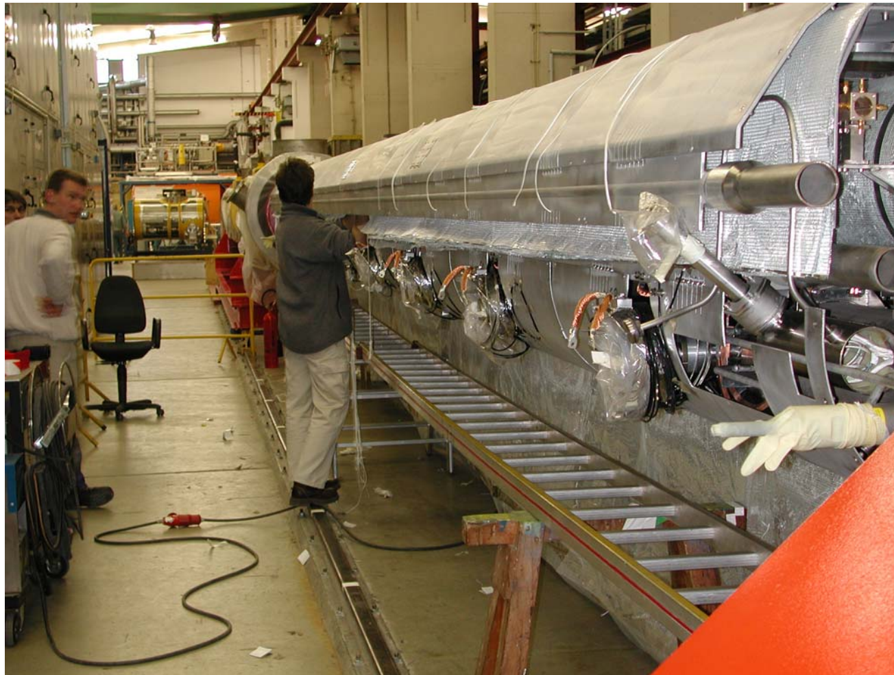
Close internal shield MLI
