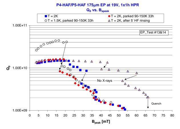
Cavity was EPed again at 17V, 25A in current control mode but the cathode bag was placed reversed and the test at 2 K showed Q-disease.
