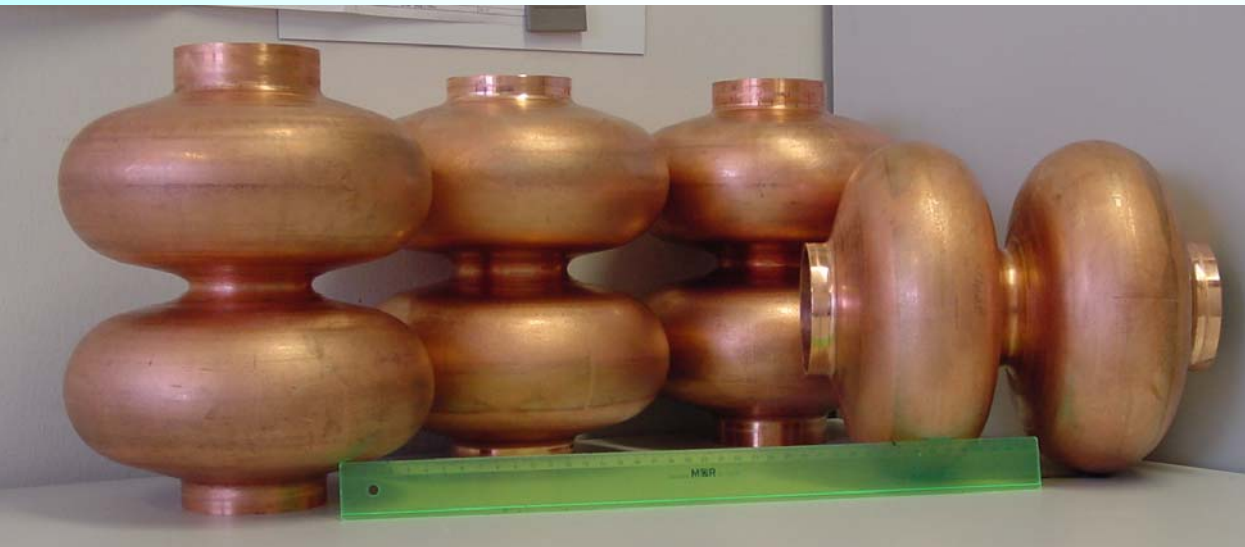
First four 2-cell NbCu clad cavities recently produced at DESY from four KEK tubes
