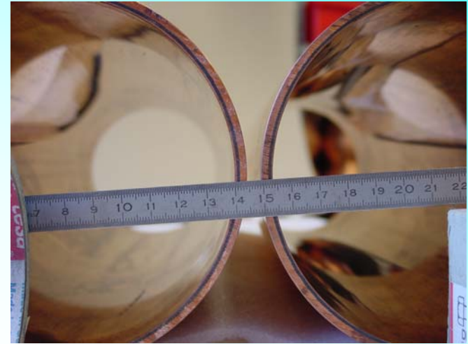
Hot roll bonded Cu-Nb-Cu tube Nippon Steel Co. and KEK
