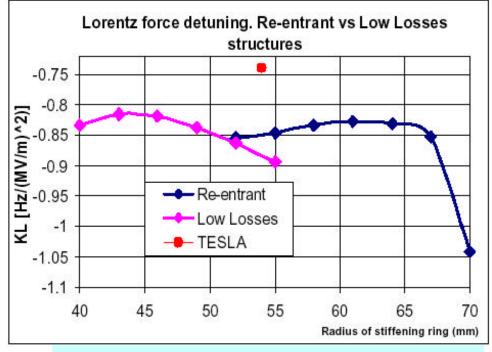
TESLA(wall=2.8mm)  $\Delta$ F(wo/w ring) = -801/-463 Hz for 25 MV/m Low Losses(2.8mm)  $\Delta$ F(wo/w ring) = -871/-509 Hz for 25 MV/m Re-entrant(2.8mm)  $\Delta$ F(wo/w ring) = -860/-517 Hz for 25 MV/m
