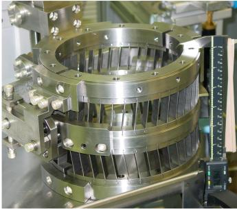
Blade Tuner range 0.3 mm without load.
