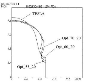
Opt $_70\_20$  - reentrant cavity with aperture 70 mm, electric field 20 % higher than in TESLA, magnetic field 10 % less than in TESLA, at the same acceleration.
