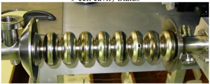
First cavity was finished but last EB welds was failed (see hole at equator). Will be repaired at JLAB. Second cavity under building now. Next 4+1 3<sup>rd</sup> harm cavities is planning to build this year with help of JLAB.
