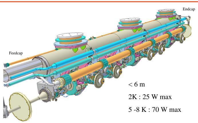
Cryomodule Main Elements Assembly on HeGRP
