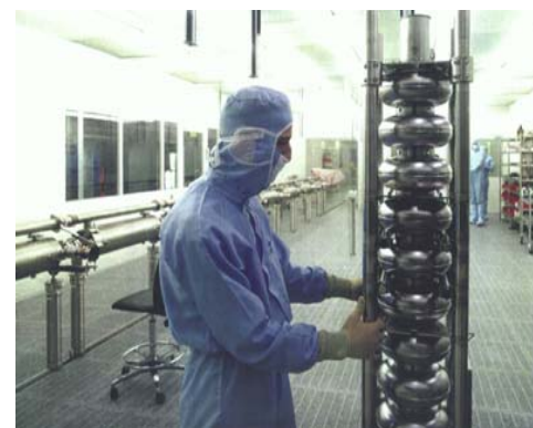
Cleanroom handling of niobium cavities
