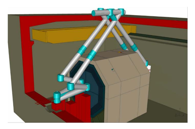
For easier manipulation with bridge crane and smaller vibrations it may be better to hide the laser tubes under the detector
