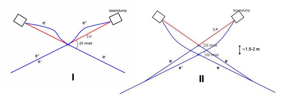
The scheme II looks attractive. The angle for  $e^+e^-$  and  $\gamma\gamma$  are different. The required shift of the detector is not a problem (the beam dump is the same).
