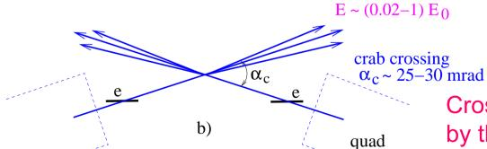
Crossing angle is determined by the angular spread in the disrupted beam and the radius of the first quad
