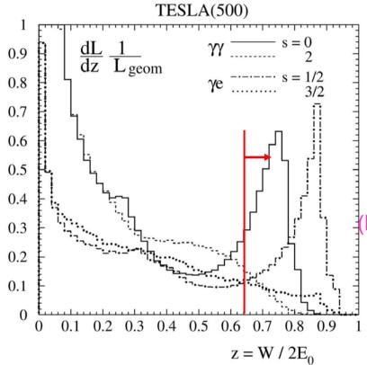
Usually a luminosity at the photon collider is defined as the luminosity in the high energy peak, z>0.8z<sub>m</sub>.
