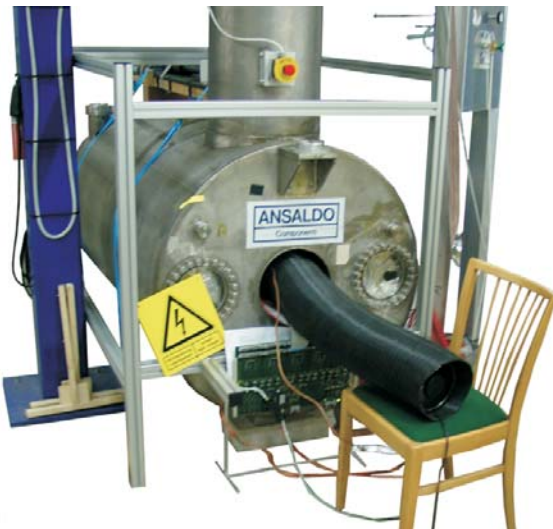
DESY 5.5T magnet, cosmics => small diffusion TDR gas at 4T as in TESLA-TDR, only short drift distances
