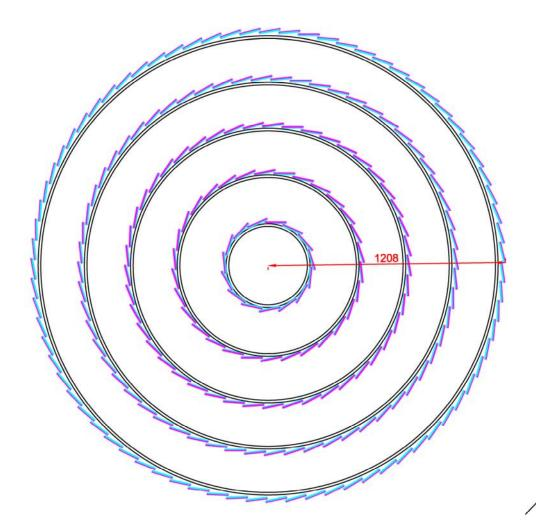
Sensors: Cut dim's: 104.44 W x 84 L Active dim's: 102.4 W x 81.96 L Boxes: Outer dim's: 107.44 W x 87 L x 4 H Support cylinders: OR: 213.5, 462.5, 700, 935, 1170 Number of phi: 15, 30, 45, 60, 75 Central tilt angle: 10 degrees Sensor phi overlap (mm): Barrel 1: 5.3 Barrel 2: 0.57 Barrel 3: 0.40 Barrel 4: 0.55 Barrel 5: 0.63 Cyan and magenta sensors and boxes are assumed to be at different Z's and to overlap in Z. Within a given barrel, cyan sensors overlap in phi as do magneta sensors.
