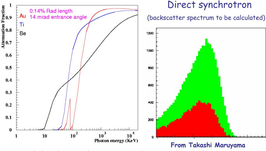
Liners help taking out low energy synchrotrons, but is the attenuation adequate for high energy synchrotrons?
