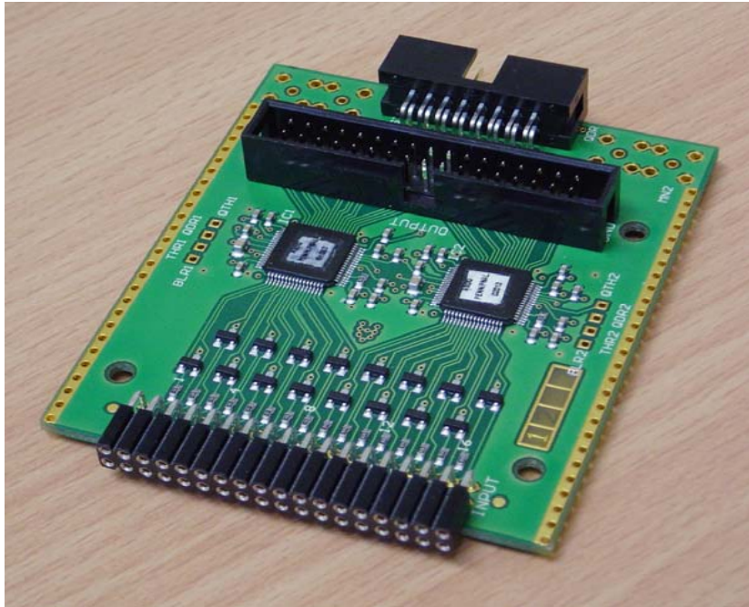
16 channel ASDQ board: preamplifier and charge-to-time converter
