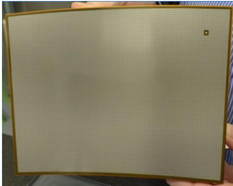
Mesh on top of a charge-dispersing resistive anode
