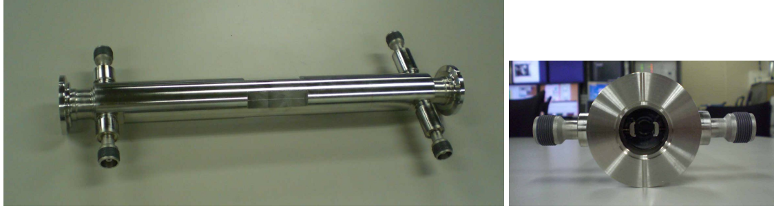
Figure 46: Side view of the stripline kicker
