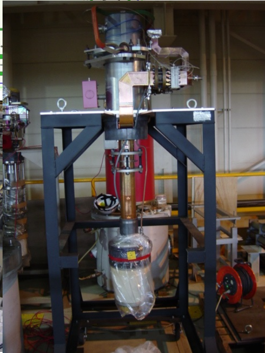
This 80MW klystron (TOSHIBA) is widely used for other accelerators, Spring8(Japan), PAL(Korea),... but only for ATF at KEK.
