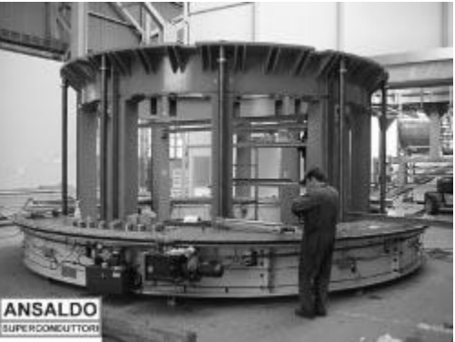
Winding table : A fixed table supports a rotating table. Both tables can move in vertical position (through the large rods attached to the central structure),
