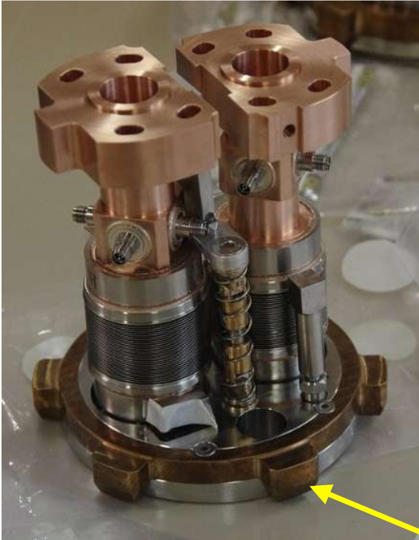
BPM-bellows tubes (about 14 cm long) set on a lock flange for RVC
