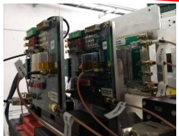
Figure 8.12: Seven 17" silicon ASIC modules, equipped with SKIROC CMS ASIC, mounted on a copper support (cooling phase during the 2017 forward campaigns). CALICE 29 mar
