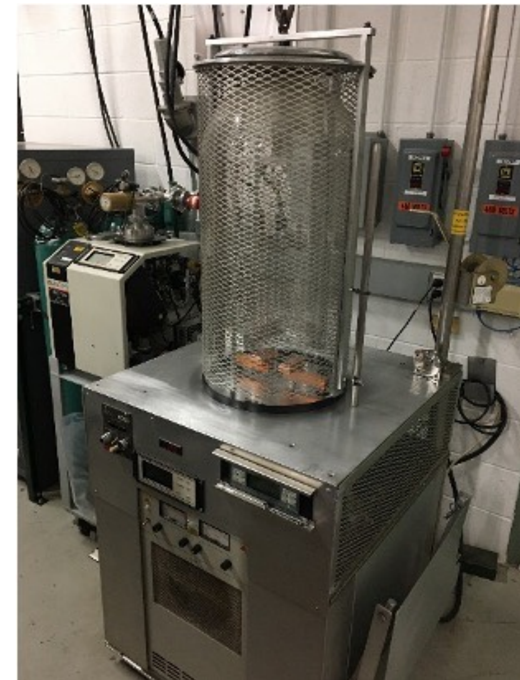
Fermilab evaporation system for CsI photocathode deposition
