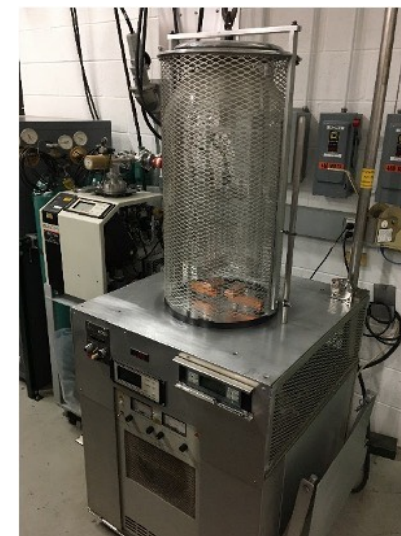
Fermilab evaporation system for CsI photocathode deposition
