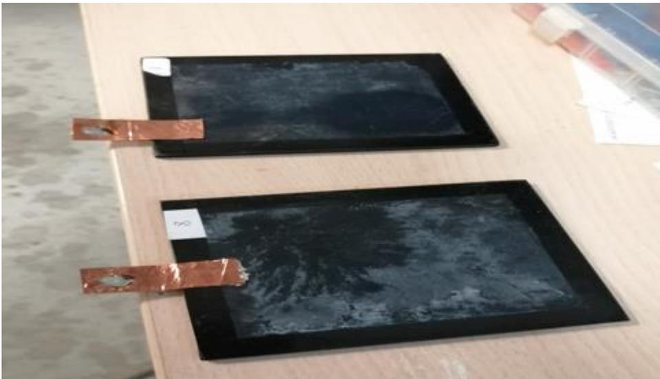
A few small detectors were made using doped PVdF plates of 2-3 mm thickness.
