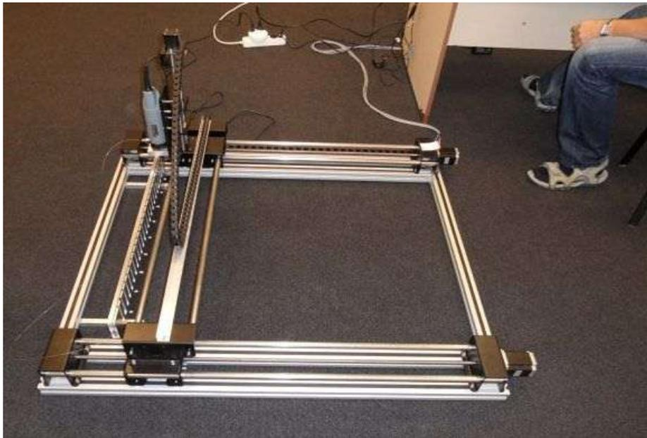
Alu/PCB Template with moving scintillator tile
