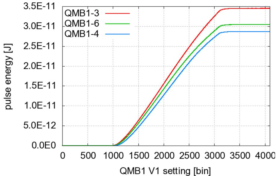
Output optical power vs V1 setting,
