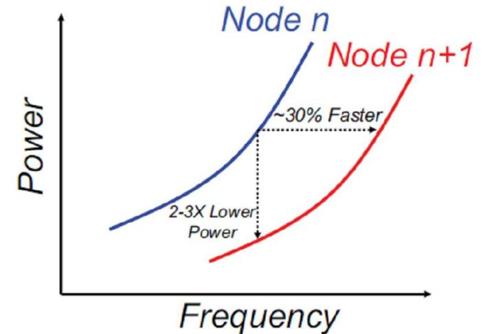
Fig. 2. Historical value of scaling: Moving to node (n+1) from node (n), and operating at lower voltage, one could obtain faster and/or at lower power.
