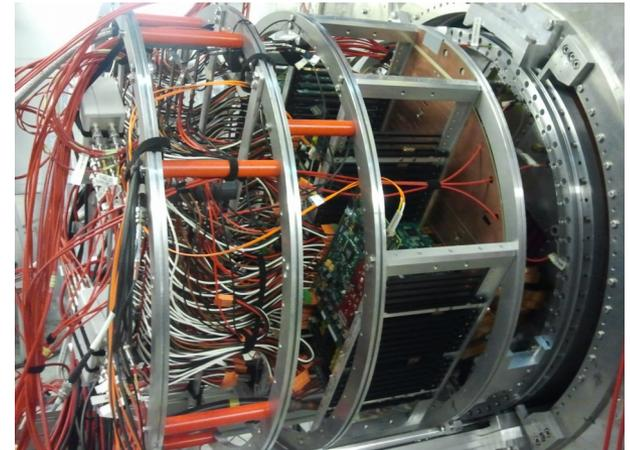
Electronic boards installed and connected to the modules
