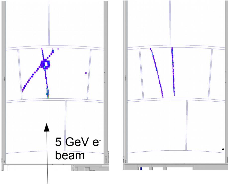
Event displays with a single module installed in the Large Prototype
