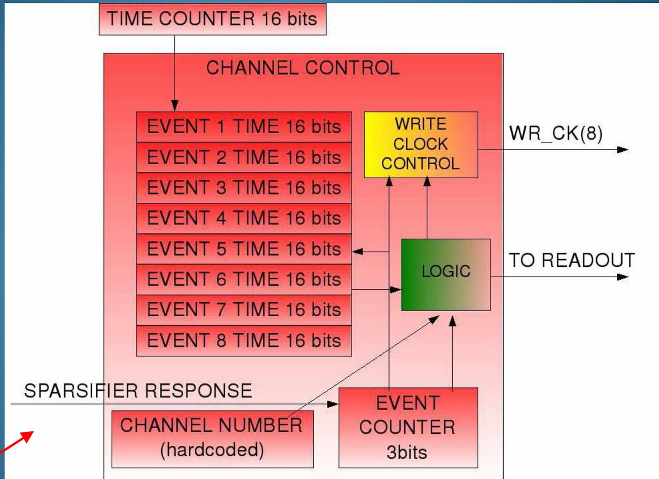
**Channel control:** inside every channel logic there are 8 registers to store the samples time information and a 3 bits event counter
