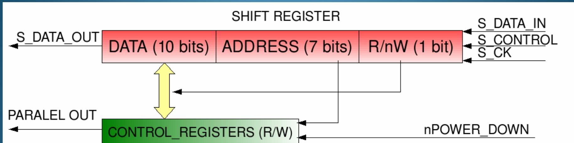
The control and configuration interface block uses a serial interface to read or write values to/from internal registers
