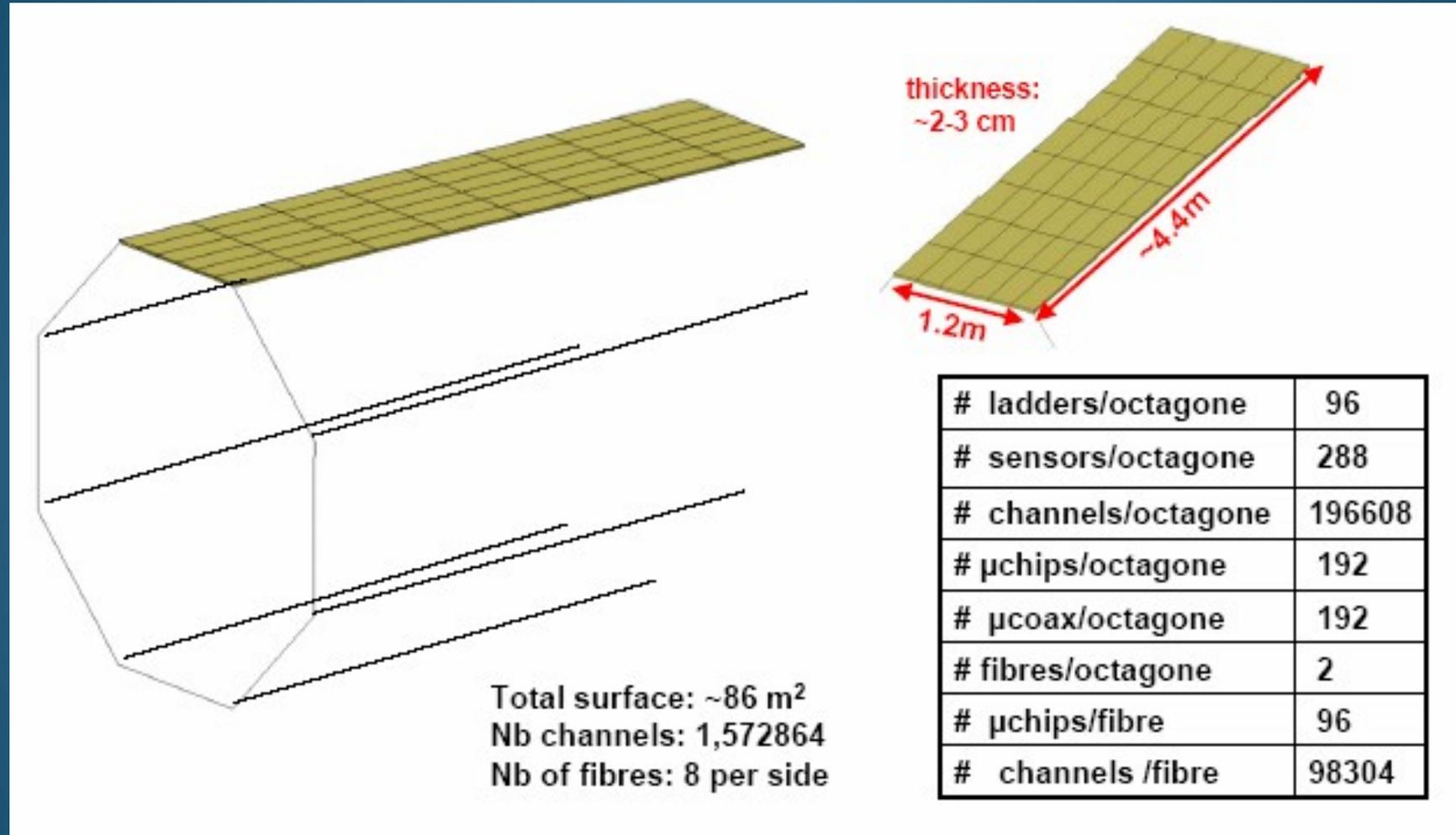
Outer Silicon tracking layer : false double sided sensors
