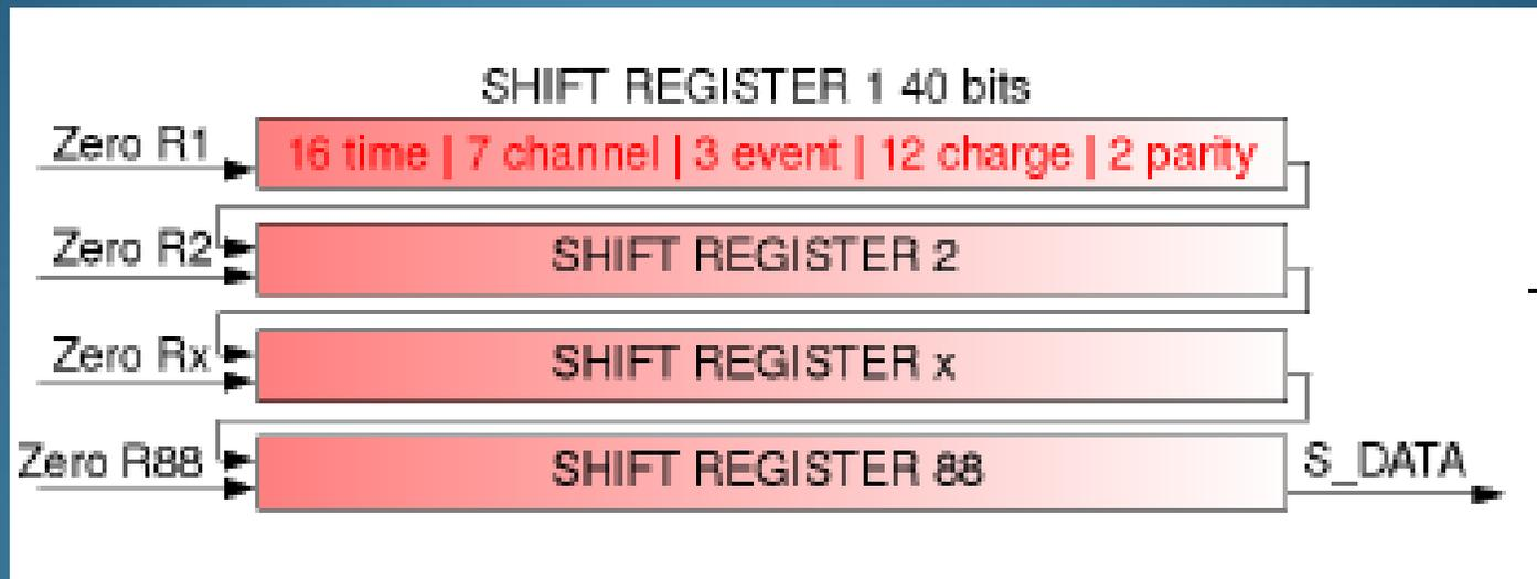
The readout block uses a serial interface to read out the data.
