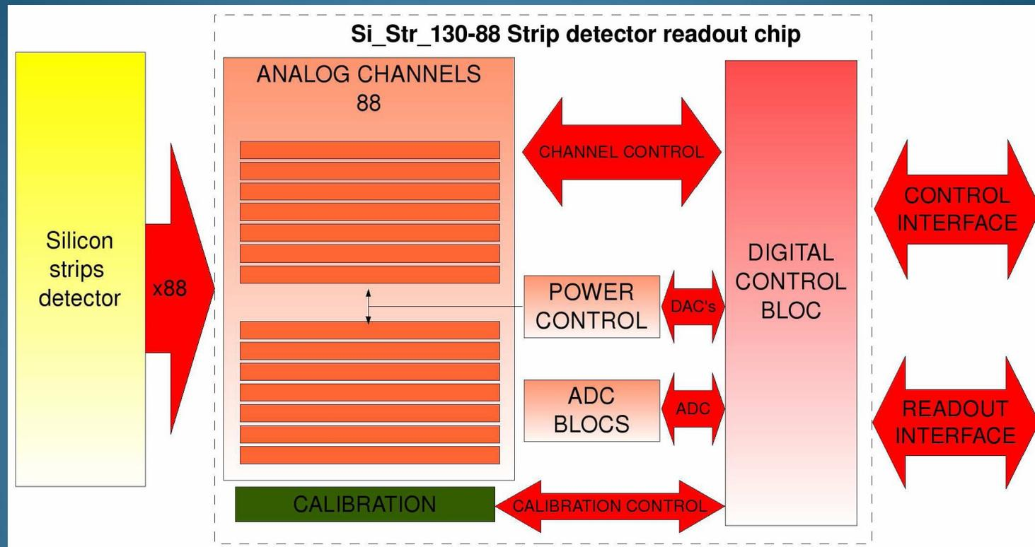
The digital part has been designed to match with the analogue part
