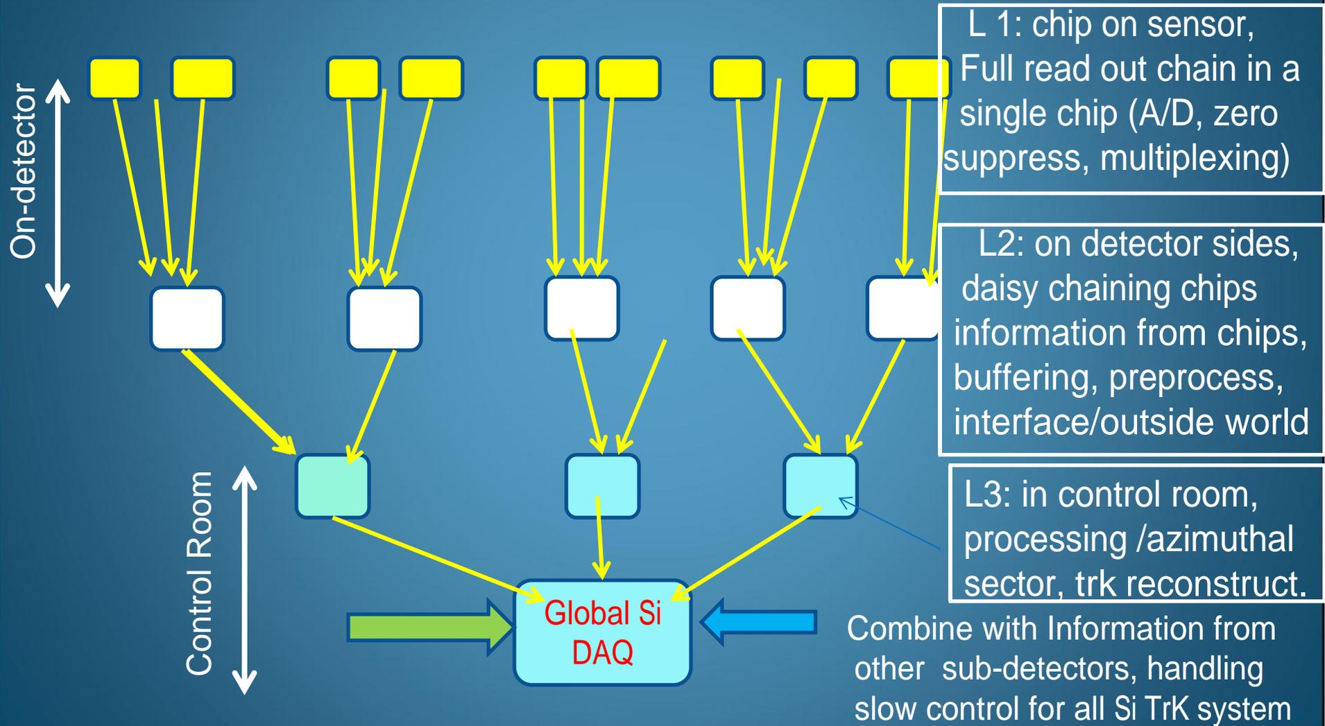
Silicon tracking DAQ Level 1:
