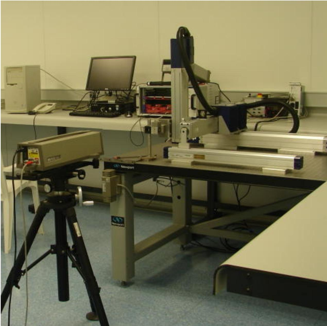
**Linearity** (comparison of reconstructed position of a fixed laser spot scanned over the sensor vs displacement of motors) will be studied using a 3D motion table.
