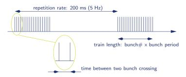
Additionaly, the front end is shut down during inter-train period to save power.
