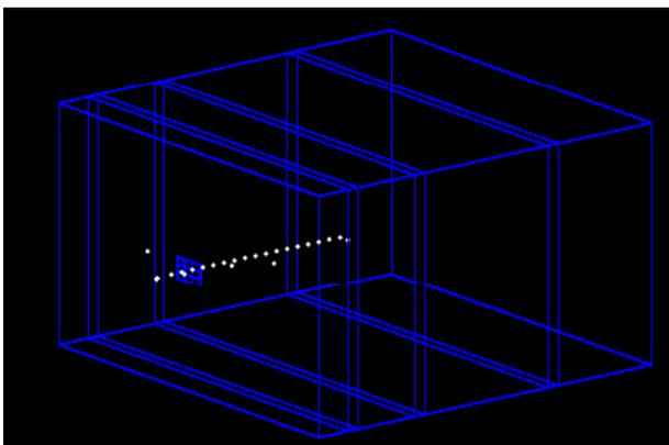
visible energy deposited by a muon in 23 calorimeter layers compared to true MC with and w/o digitization.
