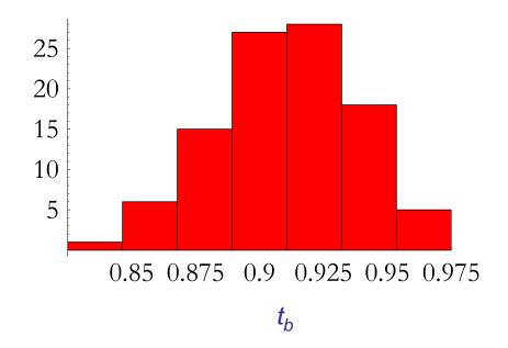
• Remember: beam turn-on time is  $T_b \ln(2)$ , and  $t_b = T_b / \tau_0$ ,  $\tau_0 = 2Q_0 / \omega$ , with  $Q_0$  the matched loaded Q at G= 34 MV/m
