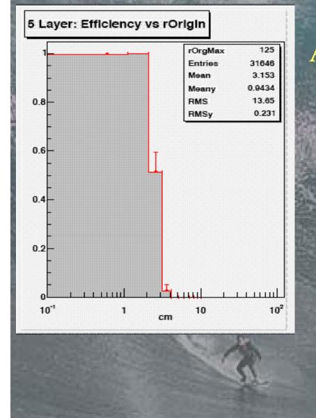
About 5% of tracks originate outside the 2<sup>nd</sup> layer of the VXD. Is the SiD able to reconstruct these?
