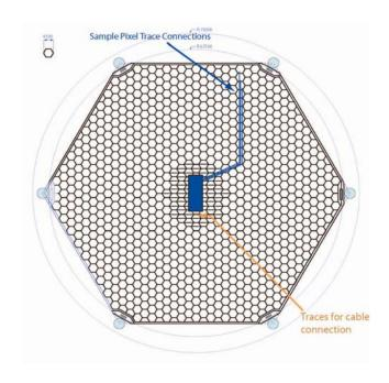
$O(1000 \text{ m}^2)$  silicon 80 million channels Pixel size ~  $13 \text{mm}^2$
